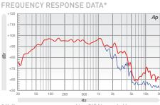
\* Half space response measured in a 965 litre sealed box Blue Line = fundamental 45° off-axis
